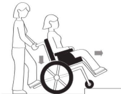
Figure 5.1: Assistant position for climbing curbs, for wheelchair with step tubes
