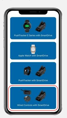
3. Connect to the SmartDrive and verify Control Configuration is set to 'Wired Controls'.
