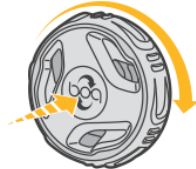
Push to engage the system Turn right to tighten
